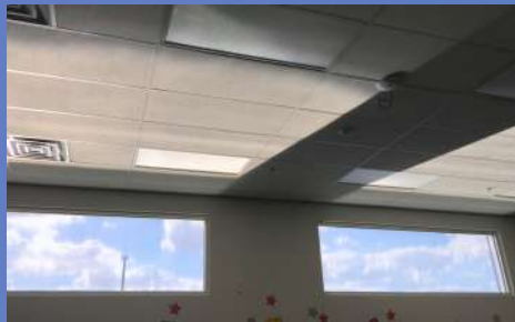
Glare is redirected towards the ceiling which then converts it into beneficial daylight, illuminating the space below.
